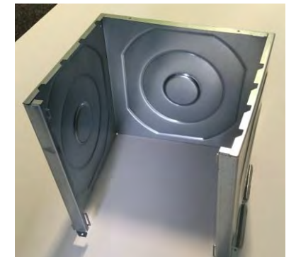
Ventilation box DC01, t_0 = 1,0 mm
