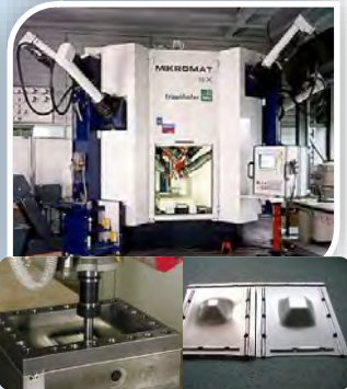
2004: Basic studies using the Mikromat 6X parallel kinematic milling machine
