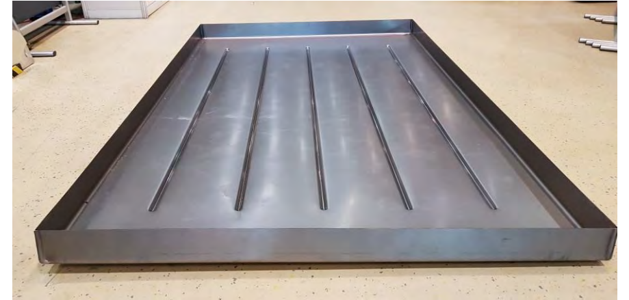
Beaded plate 2.500 mm x 1.500 mm DC01, t_0 = 1,5 mm
