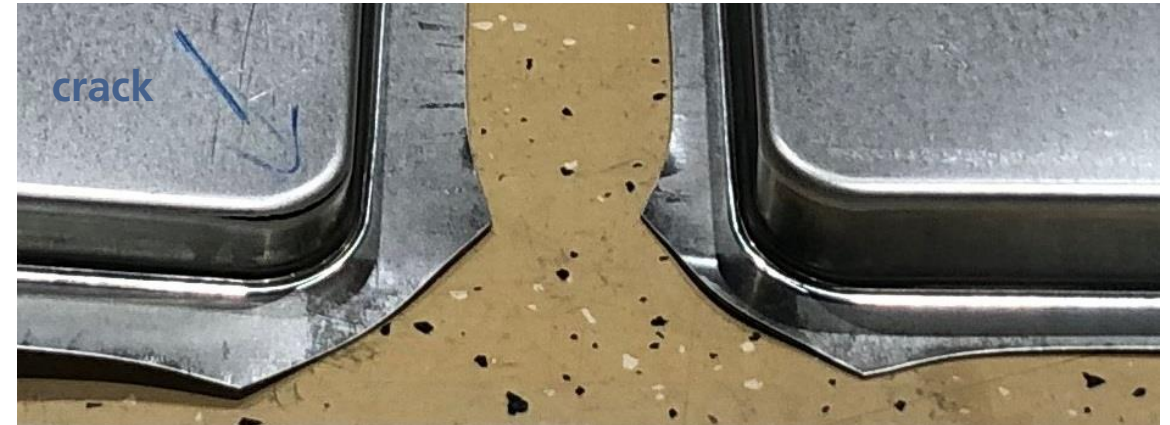
Deep drawing 20,5 mm with crack
