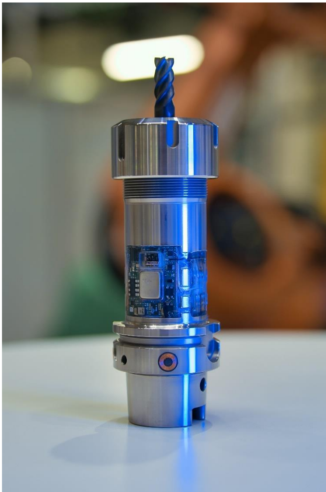
Fig. 3 The tool holder smartTOOL is equipped with sensors for measuring vibrations, process forces and temperature.
