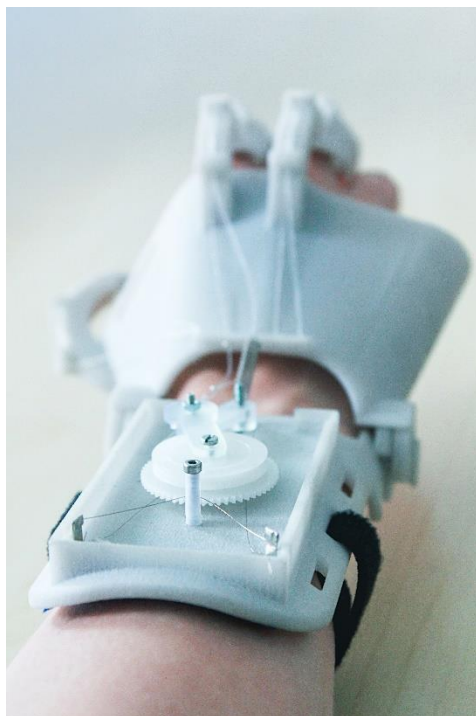
Fig. 2 The stepper drive includes gear, lever, pawl, and SMA wire components. © Fraunhofer IWU
