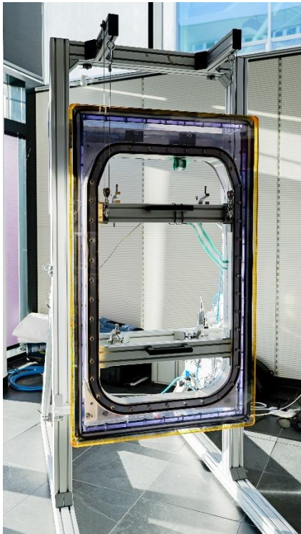
Fig. 5 Fraunhofer LBF developed and validated experimental measurement technology for sensor-integrated aircraft door seals in the TAVieDA project; project partner Trelleborg developed the new sealing geometry with, for instance, the help of finite element simulations. In this process, the component under consideration is virtually divided into a limited number of small, simple geometric elements (finite elements). © Fraunhofer IWU
