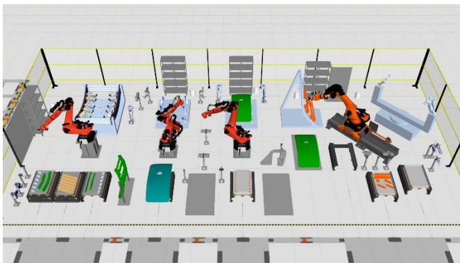
Fig. 1 Screenshot (Video available online): Fully automated assembly/joining processes and logistics for the door structure. © Fraunhofer IWU
