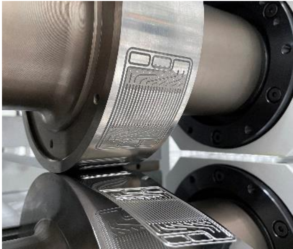
Fig. 2 The main advantage of hollow embossing is its continuous process, enabling high throughput at low costs. The image shows Bipolar plate production with BPPflexROLL. © Fraunhofer IWU
