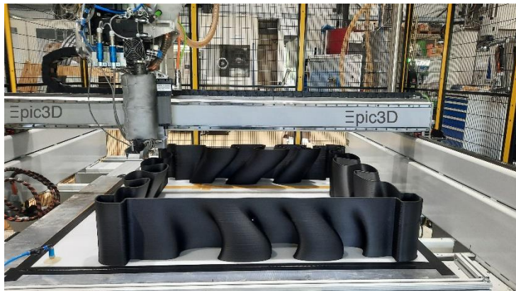
Fig. 1 The new portal printer Epic3D enables the additive manufacturing of large-size components. © Fraunhofer IWU
