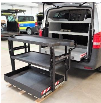
Fig. 5 Fraunhofer IWU and MOSOLF Special Vehicles GmbH have developed a 3D-printed rear shelf that, in the case of the Mercedes Vito, reduces weight by 26.5 kilograms compared to the previous retrofit solution, including the hardware. Despite this weight reduction, the payload capacity of the shelf system remains fully preserved. The shelf, printed using the SEAM process, fits seamlessly against the vehicle's outer skin, requiring no additional reinforcements or fasteners, thus making optimal use of the available space in the rear area. The two partners are also working on other interior components for special vehicles, notably interior partitioning systems. © MOSOLF Special Vehicles GmbH
