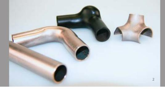
SHF has a high potential for economic efficiency, especially for small quantities, since only one component-specific die is required for production and no shaping punch is needed. By combining SHF with further processes and especially by integrating joining operations, it becomes more economical than ever to produce components and assemblies.
