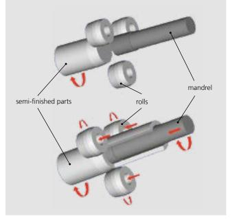
materials. Compared to impact extrusion, spin extrusion is advantageous, especially when generating thick-walled hollow parts or parts with steps. Generally, this is valid for diameterwall thickness ratios of D:s < 5. Furthermore, spin extrusion does not require chemical pre-treatment of the surface. Due to kinematic shaping this process is highly flexible, making elaborate dies unnecessary. Its economical feasibility thus extends as well to small batch manufacturing.
