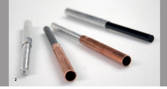
Due to the contact-free force application, the applied inductor is associated less strictly to the part geometry, compared to conventional forming tools. Provided that part geometries and especially the dimensions of the cavity that is to be formed are similar, the coil need not be exchanged. For shaping defined geometries different strategies were tested at the Fraunhofer IWU. Thereby, forming operations with single as well as multiple subsequent discharges were considered.
