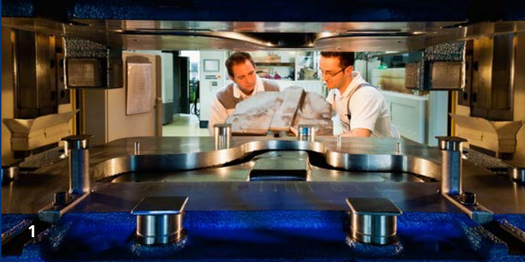
1 Test tool "B-pillar base"
