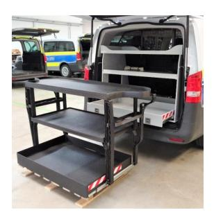
Fig. 1 The comparison with the standard shelf (installed) demonstrates the optimized space utilization of the 3D-printed model © MOSOLF Special Vehicles GmbH November 06, 2023 || Page 3 | 3
