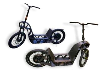
Fig. 2 DynaLight Project: Load-bearing frame construction for the electric cargo scooter from the 3D printer ©Fraunhofer IWU www.iwu.fraunhofer.de
