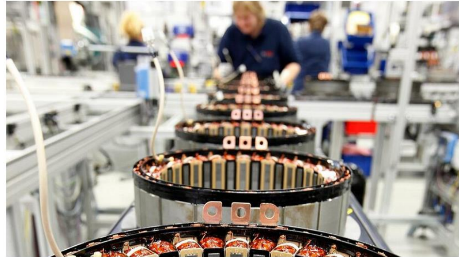
Electric motor production at Bosch Much bit fewer components than for a conventional engine
